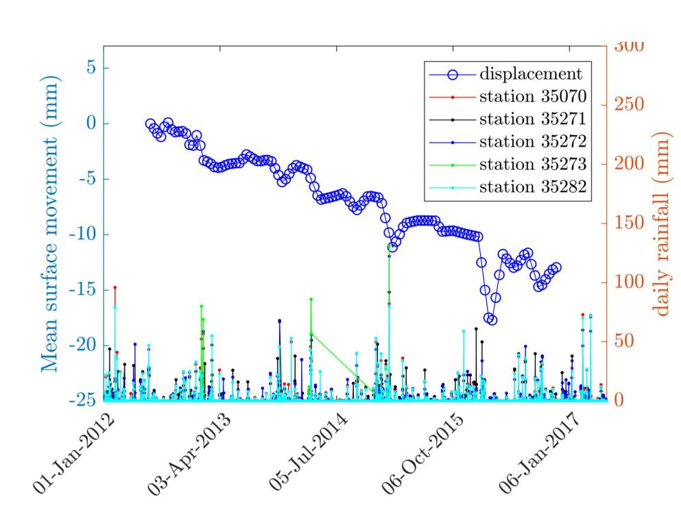
*Figure 1:* Net surface movement and rainfall near Taroom, showing a background trend of downward movement and accelerated movement during the wet season.
