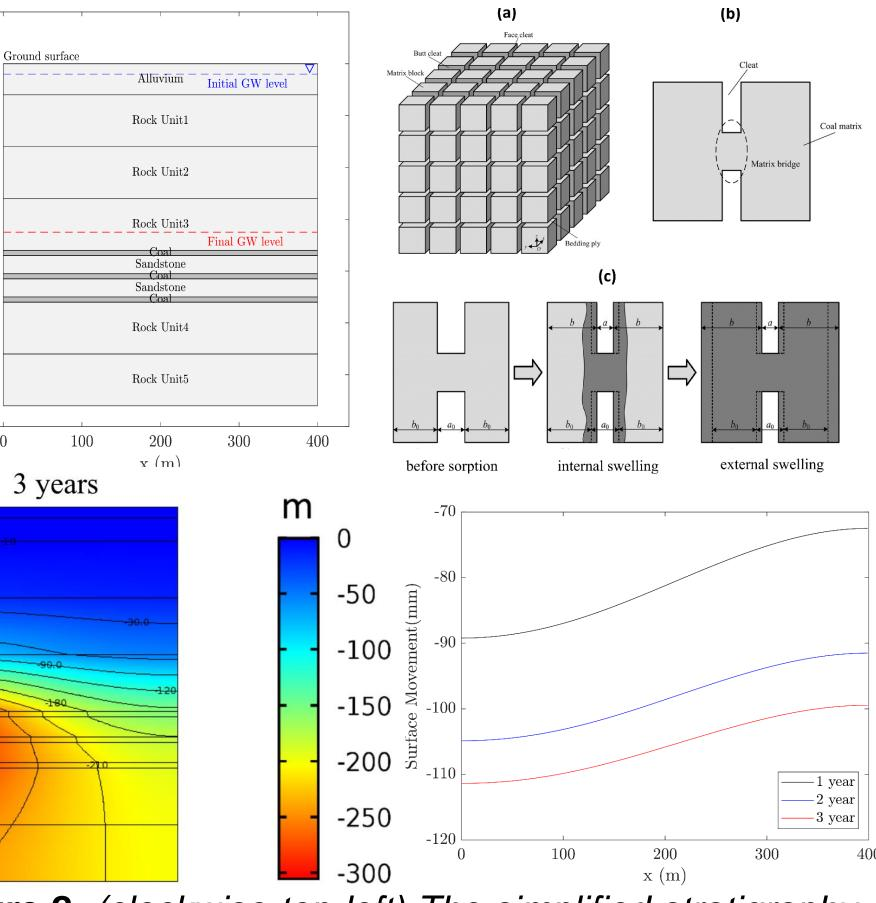
*Figure 2:* (clockwise top left) The simplified stratigraphy used in modelling; mechanisms of internal and external coal swelling, depressurisation; and surface movement.
