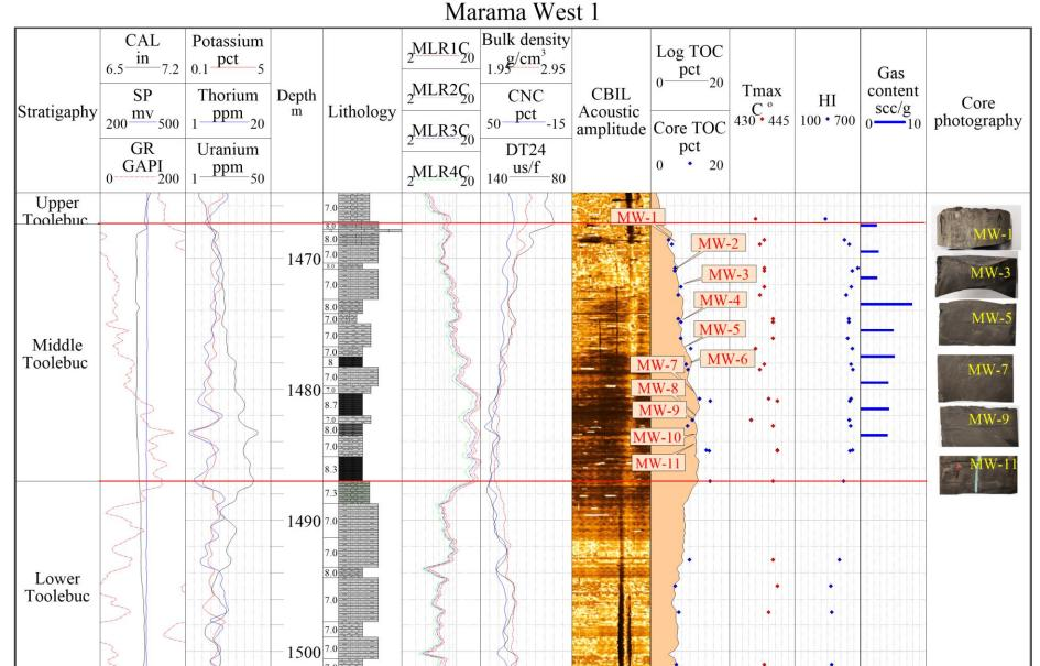
Figure 2: Wellbore logging data analysis and sample depth selection
