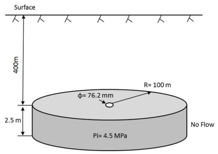
Illustration of numerical model geometry. The compositional simulator GEM from the Computer Modelling Group (CMG) suite was used. The radial grid system has **100 grid cells** in the **radial direction**, **3 grid cells** in the **angular direction** and **1 grid cell** (layer) in the **vertical direction**, making a **total of 300 grid cells** in the model.
