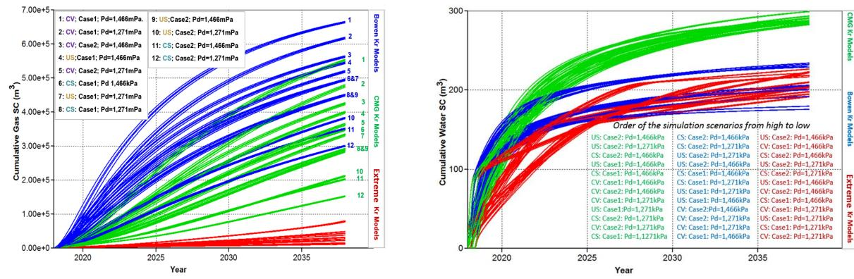
Cumulative gas production for different reservoir conditions under different dewatering rates over 20 years
