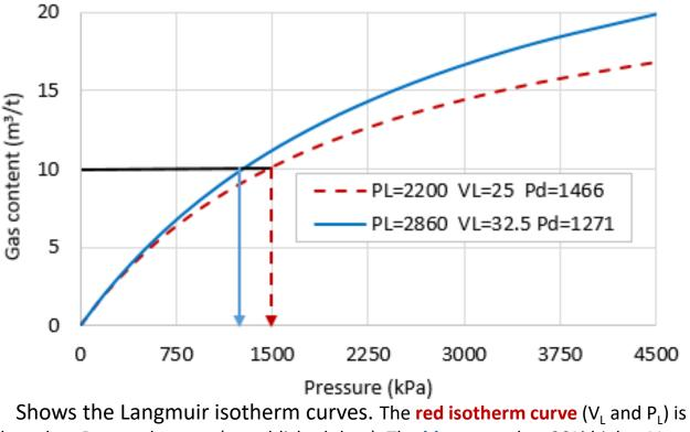
based on Bowen datasets (unpublished data). The **blue curve** has 30% higher  $V_{L}$  and  $P_{L}$ . Both curves were calculated with gas content GC=10 m<sup>3</sup>/t
