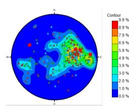
(b) Stereonet contour of faults and fractures dip azimuth in Waukivory12 well
