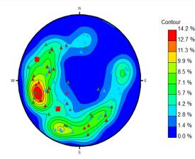
Stereonet contour of faults and fractures dip azimuth in Waukivory11 well
