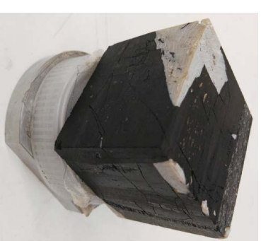
40 mm cubic coal sample
