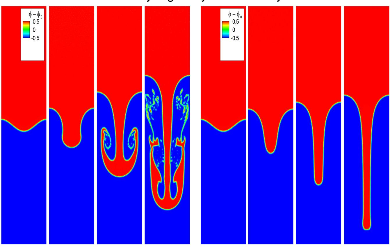
Base case (left) has a density ratio of 3 for comparison to previous works, extension case (right) has water-air-like properties.
