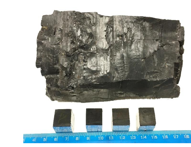
Fig. 2 Sub-bituminous coal cubes from Surat Basin (Dimension of 15 mm)
