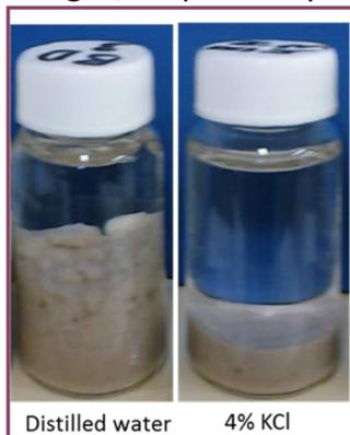
Figure 1. Illustration of visual swelling test method
