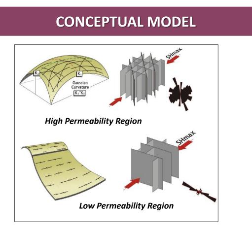
*Figure 2 In situ stress and fracture orientation with permeability (Flottman et. al 2013)*
