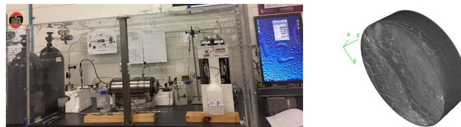
Fig. 3 Coal stimulation rig and CT Scanning Image
