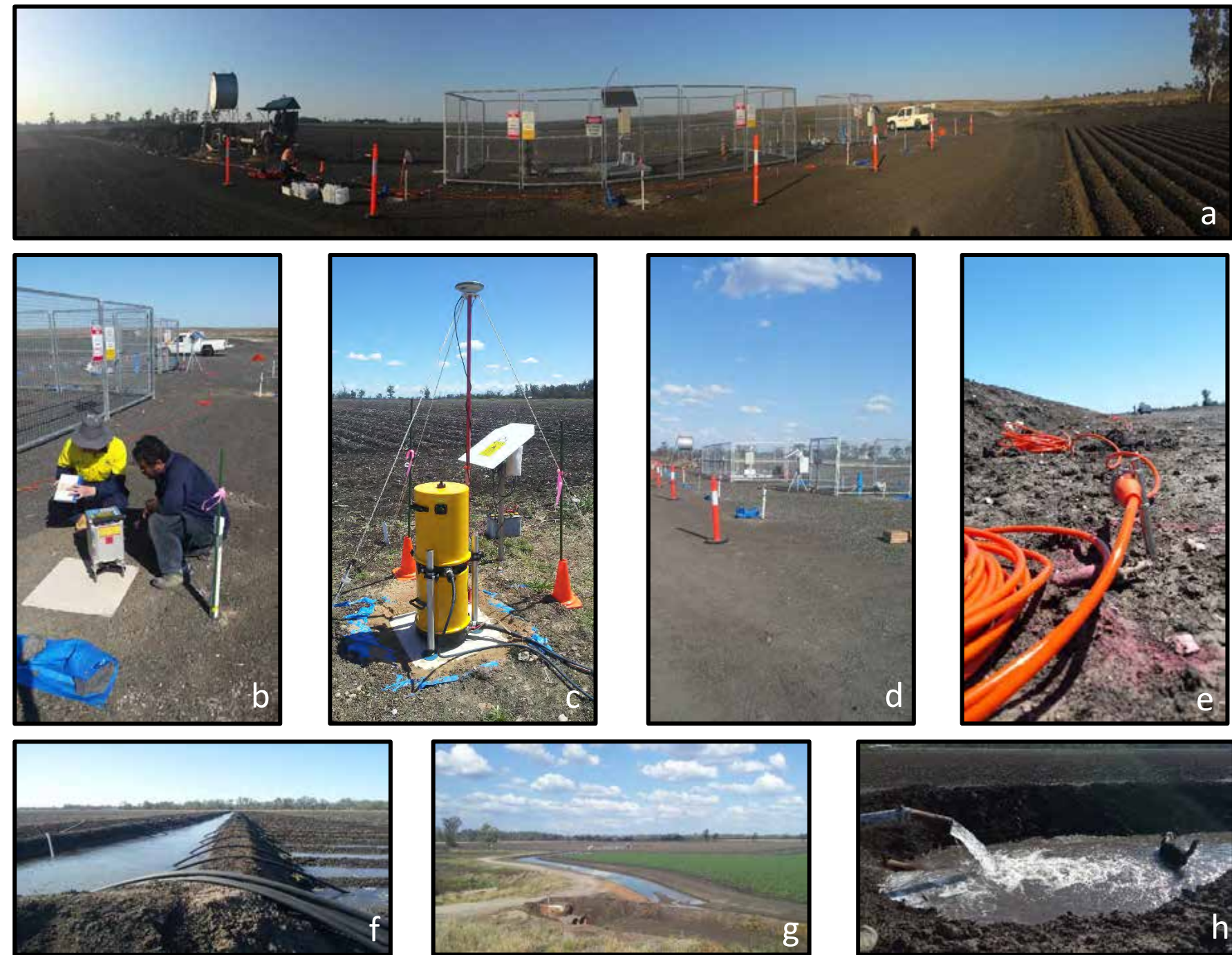
Fig 6 (a) 180° image of survey site with the farmer's diesel engine and tank for the irrigation pump on the left; enclosed monitoring wells and geophysical field equipment to the right. (b) relative gravity measurements using a CG-5 instrument; (c) absolute gravimeter A-10, on loan from Geoscience Australia and GPS base station; (d) field site; (e) resistivity cable and electrode; (f) irrigation channel and tubes to flood the paddocks; (g) landscape view of field site with irrigation channels and paddocks; (h) water pumping from the Condamine Alluvial Aquifer and Molly, the farmer's dog, taking a bath.
