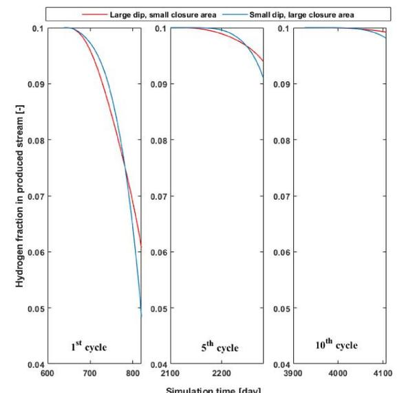
**Figure 4:** Hydrogen fraction in produced stream profiles during 1<sup>st</sup> (left); 5<sup>th</sup> (middle); 10<sup>th</sup> (right) cycle; injected hydrogen fraction is 0.1.
