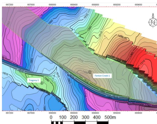
**Figure 1:** Areal view of contour map of Fenton Creek gas reservoir, the origin of structure model and data; the gas reservoir region is shaded in grey and the Fenton Creek-1 production well is marked by a cross.
